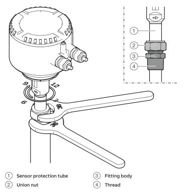
Figure 4: Tighten sensor
