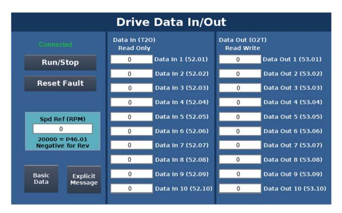
The values that appear in the Data In registers are controlled by parameter group 52 in the drive. Setting 52.01 to 1.11 would cause the DC bus voltage to appear in the Data In 1 value shown above. Setting group 52 to the drive parameters you need to use on a regular, frequent basis within the UniLogic program will cause those parameters to be transmitted to the panel at the RPI rate defined in the scanner.
