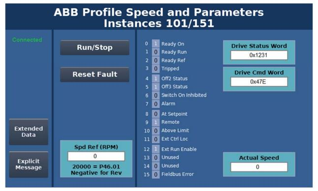
The drive should run by pressing the Run/Stop button. Speed is controlled by the Spd Ref pushbutton. A value of 10,000 will result in half speed of the motor as set by parameter 46.01 and the limits in group 30. A value of 20,000 is full speed in the ABB profile, a negative value of -20,000 will result full reverse speed.
