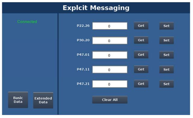
This screen demonstrates the use of low frequency, on demand use data. This is done outside of the normal messaging between the drive and UniStream using the EIP Get and Set function blocks which appear in a program as:
