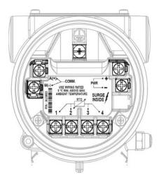
Figure 7: MODBUS Electrical Connection
