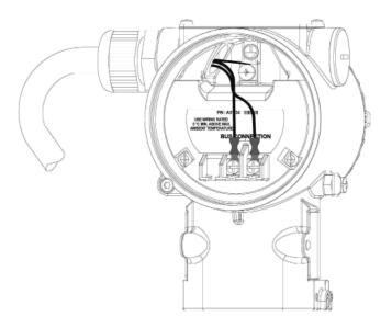
Figure 6: 266 PROFIBUS PA / FOUNDATION Fieldbus terminal block
