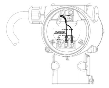
Figure 5: 266 HART terminal block
