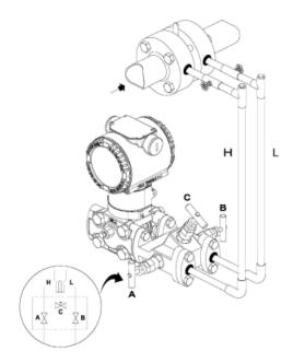
Figure 9: Steam or clean liquid flow measurement
