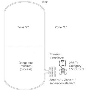
Certificate IECEx Ex d IIC T6, Ex tD A21 T85°C, Ta= -50°C to +75°C IECEx certificate number
