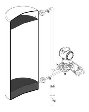
Figure 11: Level measurement on closed tank with dry leg
