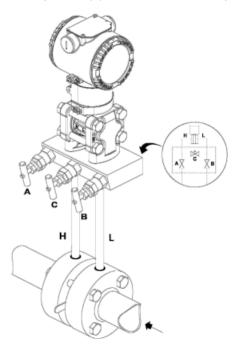
Figure 10: Gas or liquid flow measurement
