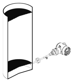
Figure 12: Level measurement on open tank with P style transmitter
