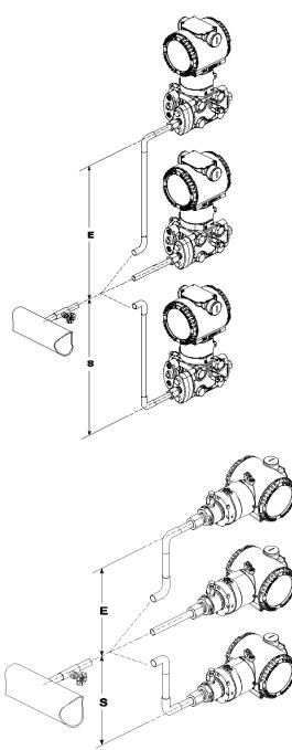
Figure 34: Gauge or absolute pressure measurement of a liquid in a pipe
