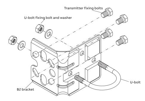
Figure 14: Pipe and wall mounting bracket kit (B2)
