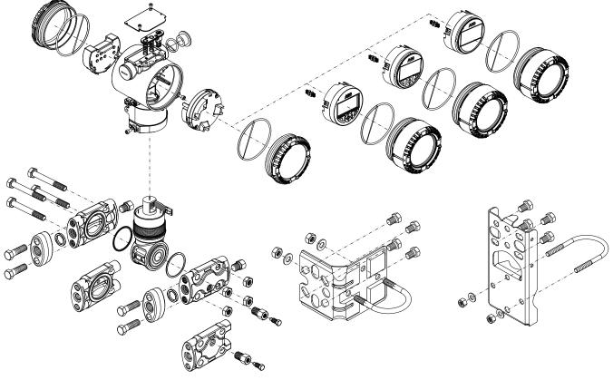
Figure 1: Differential pressure transmitter components
