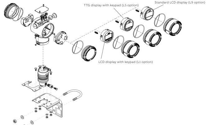
Figure 2: Gauge / absolut pressure transmitter components
