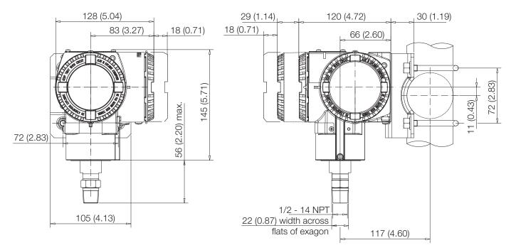
Figure 23: Model 266G or 266A P-Style transmitter with DIN housing installed on a 2"pipe with optional bracket (B2 Stainless Steel 316L)
