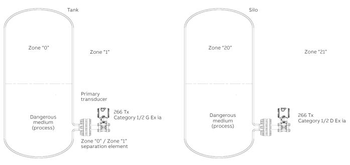
Note: the transmitter can be connected to either [ib] or [ia] supply (associated apparatus)certified [Ex ia] Note for "Primary transducer": see the certification for exceptions Note: the protection is mainly assured by the "IP" degree associated to the low power from supply. This can either be [ia] or [ib] c) Certificate ATEX II 1/2 G Ex db IIC T6 Ga/Gb and
