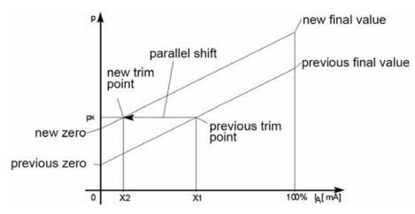
When a pressure px is applied, the transmitter displays the standardized output value x1 in percent. Due to the present application the value x2 should be displayed. Enter this new value x2 in the line PRTB\_PARALLEL\_SHIFT\_PV, the transmitter calculates the new zero and the new final value and adopts these new settings in the PRTB\_PRIMARY\_VALUE\_RANGE 0% and PRTB\_PRIMARY\_VALUE\_RANGE 100%.
