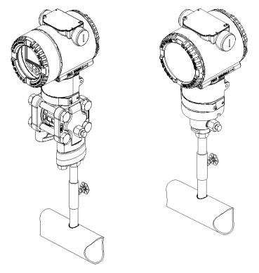
Figure 36: Gauge or absolute pressure measurement of gas in a pipe
