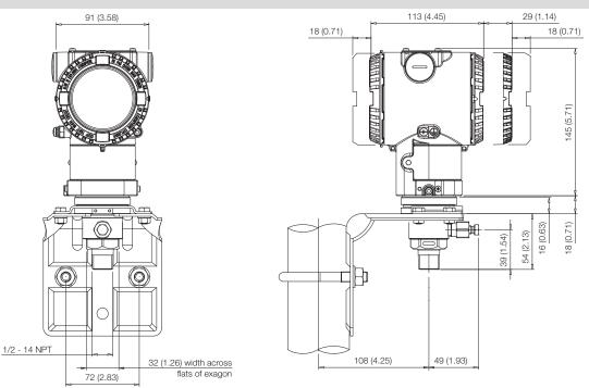
Figure 17: Model 266H or 266N High overload resistant P-Style transmitter with ½-14 NPT male process connection and barrel housing installed on a 2"pipe with optional bracket (B1 carbon steel or B2 Stainless Steel 316L)
