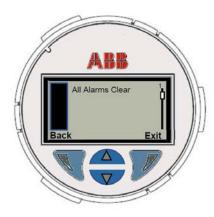
Vice-versa, when at least one error condition is active, it is displayed a corresponding error code and its source as process, sensor, electronics....
