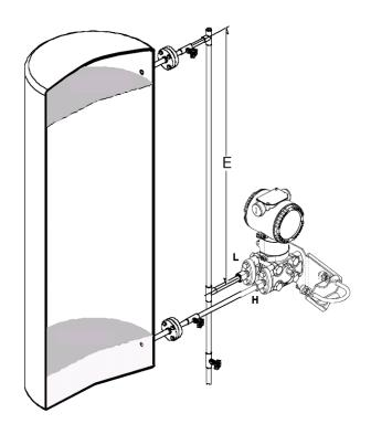
Figure 31: Level measurement on closed tank with wet leg
