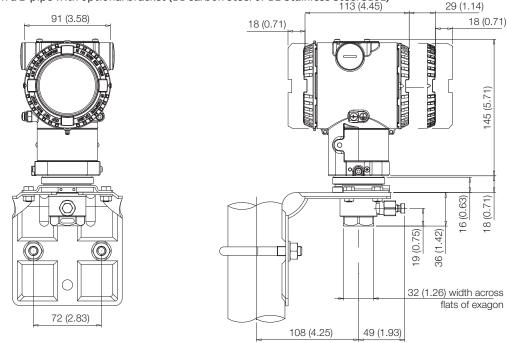
Figure 18: Model 266H or 266N High overload resistant P-Style transmitter with ½-14 NPT female process connection and barrel housing installed on a 2"pipe with optional bracket (B1 carbon steel or B2 Stainless Steel 316L)
