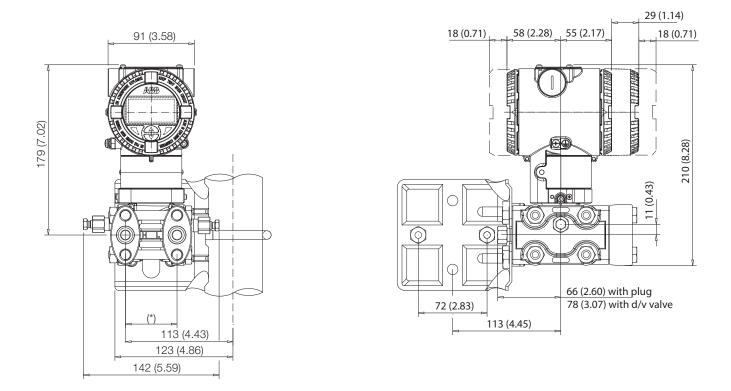
Figure 9: Differential Pressure Style transmitter with barrel housing installed on a vertical pipe with optional bracket (B2)
