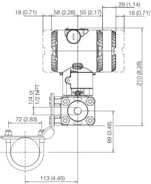
Figure 12: Differential Pressure Style transmitter with barrel housing and Kynar inserts installed on a vertical pipe with optional bracket (B2)
