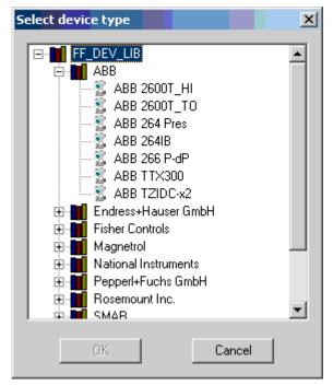
Select "ABB 266 PdP" and press OK. The 266 PdP appears now in the H1 segment with predefined TAG and Address......
