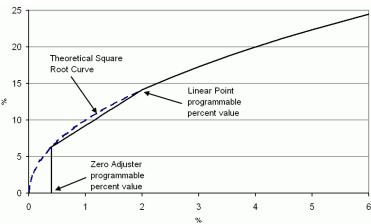
To neglect the values with the input approaching zero, the transmitter output is zero with the input up to a programmable percentage value between 0 % and 20%. This option is offer in order to ensure a more stable flow measure. This option is possible for all the listed output functions.
