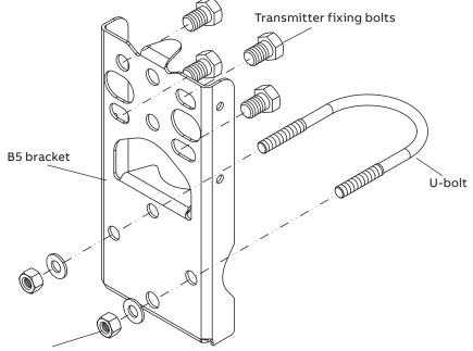
U-bolt fixing bolt and washer
