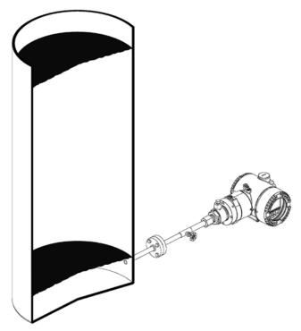
Figure 32: Level measurement on open tank with P style transmitter
