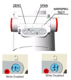
Figure 43: Pushbuttons - functionalities
