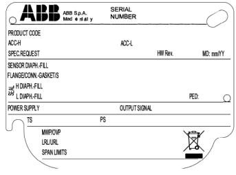
Figure 5: 266 nameplate with PED data
