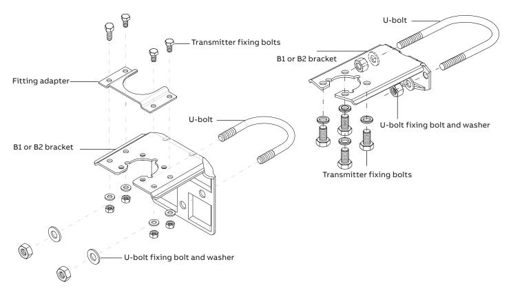
Figure 21: Pipe and wall mounting bracket kits for P style transmitter with Barrel housing
