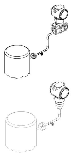
Figure 33: Gauge or absolute pressure measurement on a tank
