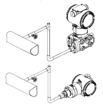
Figure 35: Gauge or absolute pressure measurement of condensable vapor
