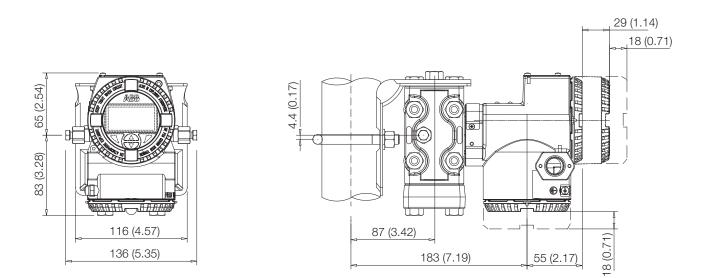
Figure 11: Differential Pressure Style transmitter with barrel housing and Kynar inserts installed on a horizontal pipe with optional bracket (B2)
