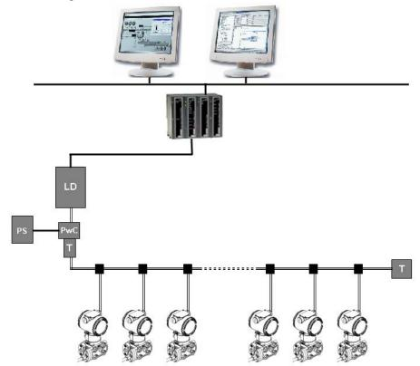
Figure 39: FOUNDATION Fieldbus architecture
