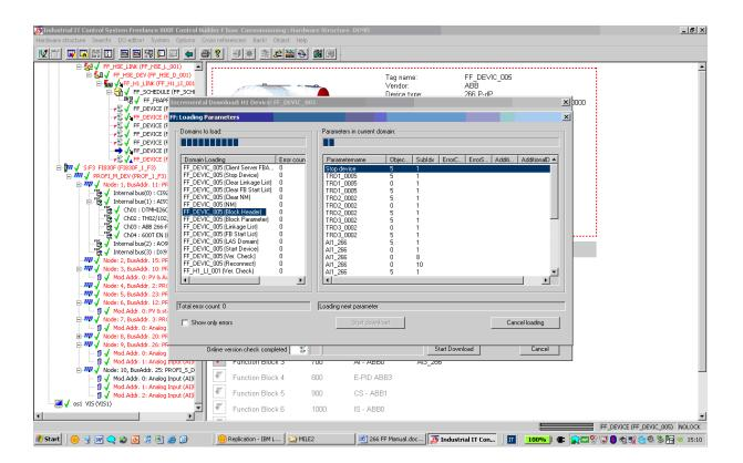
.....the transmitter's blocks used in the FBAP are moved in the AUTO or their Normal Mode.
