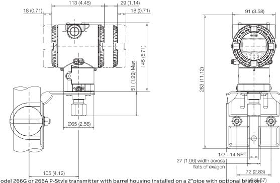
Figure 20: Model 266G or 266A P-Style transmitter with barrel housing installed on a 2"pipe with optional błacket?) (B1 carbon steel or B2 Stainless Steel 316L)
