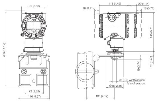
Figure 19: Model 266H or 266N High overload resistant P-Style transmitter with sensor Z with barrel housing installed on a 2"pipe with optional bracket (B1 carbon steel or B2 Stainless Steel 316L)
