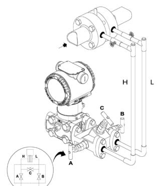
Figure 28: Steam or clean liquid flow measurement (transmitter and manifold)
