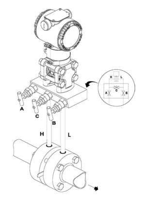
Figure 29: Gas or liquid flow measurement (transmitter and manifold)
