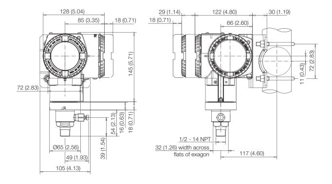
Figure 22: Model 266H or 266N Hi overload resistant P-Style transmitter with DIN housing installed on a 2" pipe with optional bracket (B2 Stainless Steel 316L)
