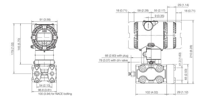
Figure 8: Differential Pressure Style transmitter (High Static option)
