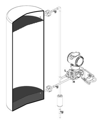
Figure 30: Level measurement on closed tank with dry leg
