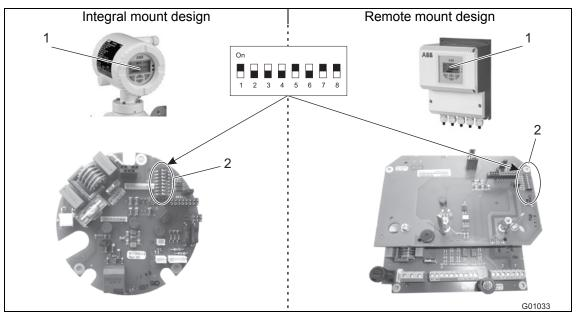
Fig. 59: Position of DIP switches
