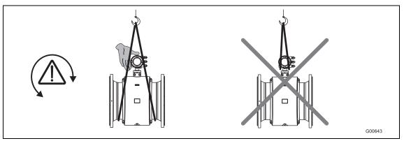
Fig. 7: Transport of flanged units smaller than DN 450
