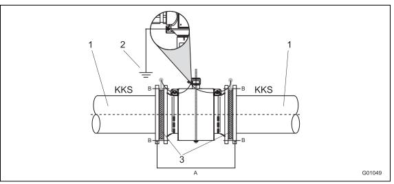
Fig. 31: Flowmeter sensor with grounding plate and functional ground
