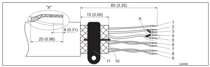
Fig. 34: Flowmeter sensor side, dimensions in mm (inch)
