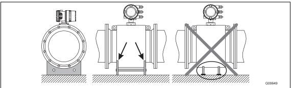
Fig. 9: Support for meter sizes larger than DN 400
