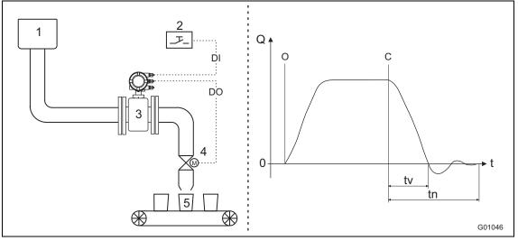
Fig. 67: Fill function (batch)
