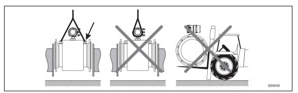
Fig. 8: Transport of flanged units larger than DN 400
