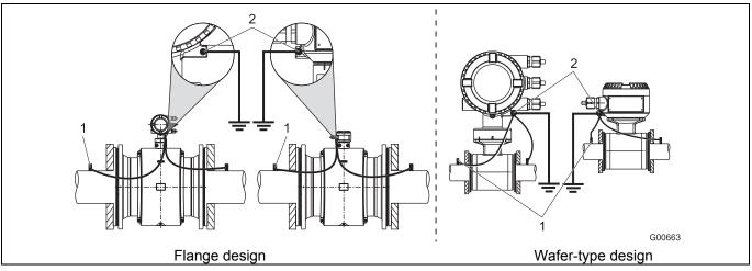
Fig. 27: Metal pipe, without liner (example)
