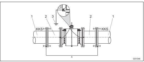
Fig. 32: Flowmeter sensor with functional ground
