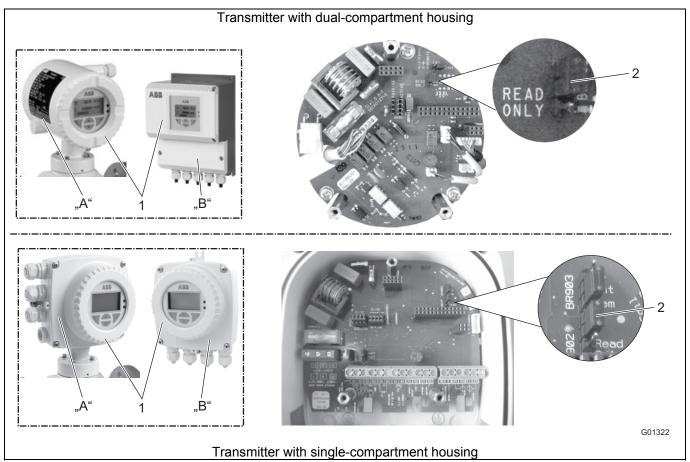
Fig. 66: Jumper for hardware write protection
