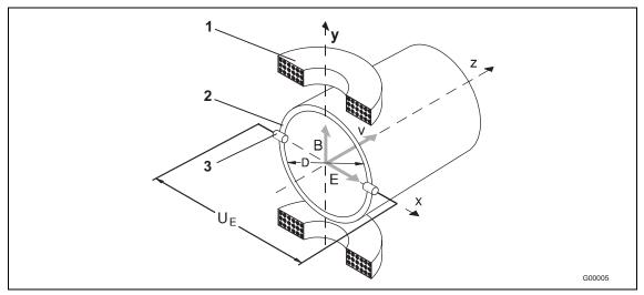
Fig. 4: Electromagnetic flowmeter schematic
