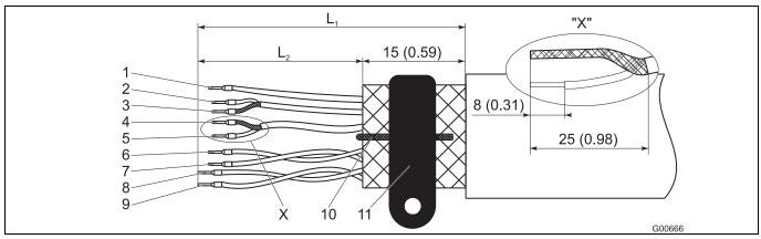
Fig. 35: Transmitter side, dimensions in mm (inch)
