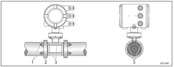
Fig. 10: Installation set for wafer-type installation
