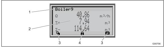
Fig. 65: Process display (example)
