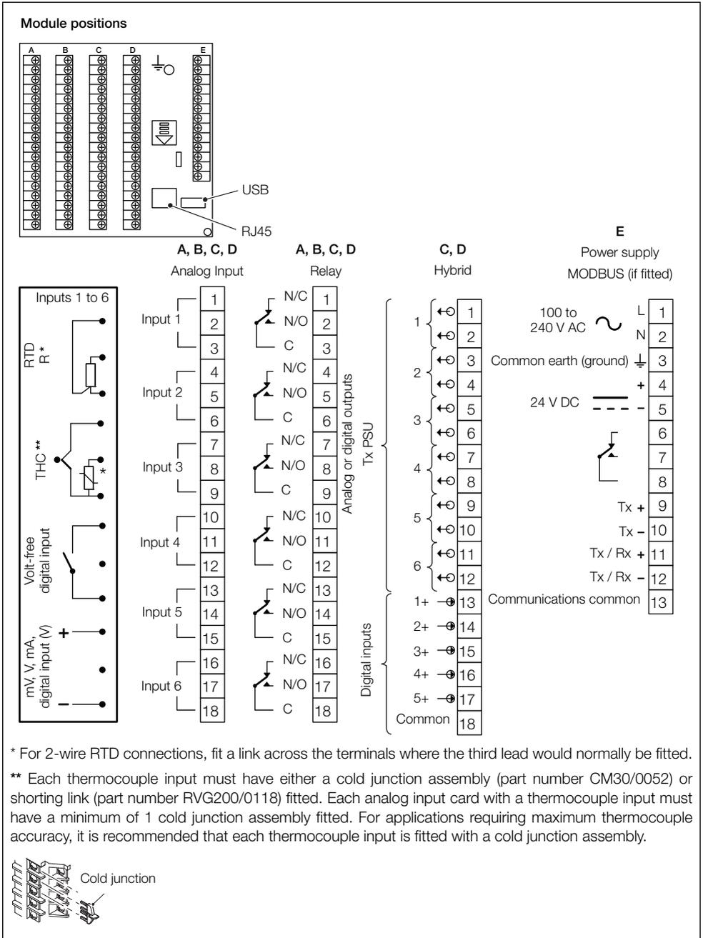
\* For 2-wire RTD connections, fit a link across the terminals where the third lead would normally be fitted.
