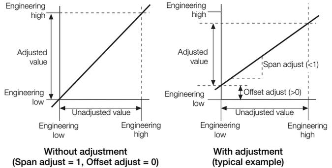
Operator Calibrate Set to On to enable input adjustment from the **Service** menu – see page 45.
