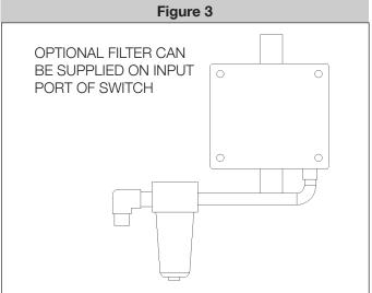
Note: The action of the pneumatic switch will be determined by user connection of Ports A, B & C. Option H or L will determine how the option filter and vent fitting are supplied from the factory. The filter and vent fitting are easily changed in the field. Reference PS45 (DS/PS45-EN) for ordering details.
