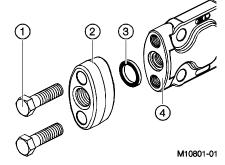
Fig. 5: Process connection 1 Screws 2 Flange adapter 3 O-ring 4 Transmitter connection flange
