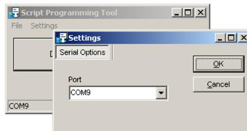
Figure 18: SPT Selection of the PC interface
