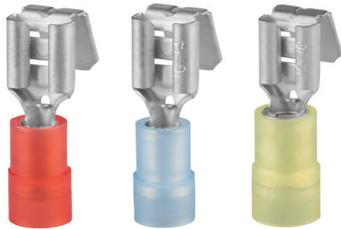
Nylon-insulated piggy back disconnects for wire termination of copper conductors ranging from 0.5mm<sup>2</sup> to 6mm<sup>2</sup>
