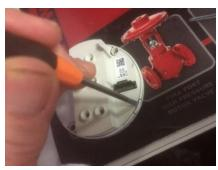
The RTD PCBA is visible after the latches are disengaged and the assembly is separated.
