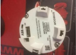
Remove the cable from the back of the module.
