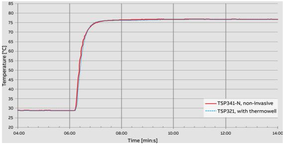
17 Temperature jump from 29 °C to 77 °C. Measuring medium: water, piping not insulated
